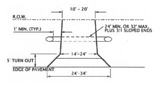
\* SIDEWALK TO BE CONTINUOUS, CONSTRUCTED SEPERATE FROM DRIVEWAY, AND SHALL CONFORM TO CURRENT ADA REQUIREMENTS
